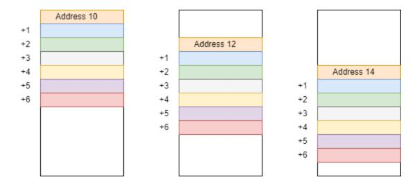
In our buffer overflow example, we know the return address is 16 bytes after our buffer. So, if we find the buffer was at address 10, the return address must be at address 26, and so on.
