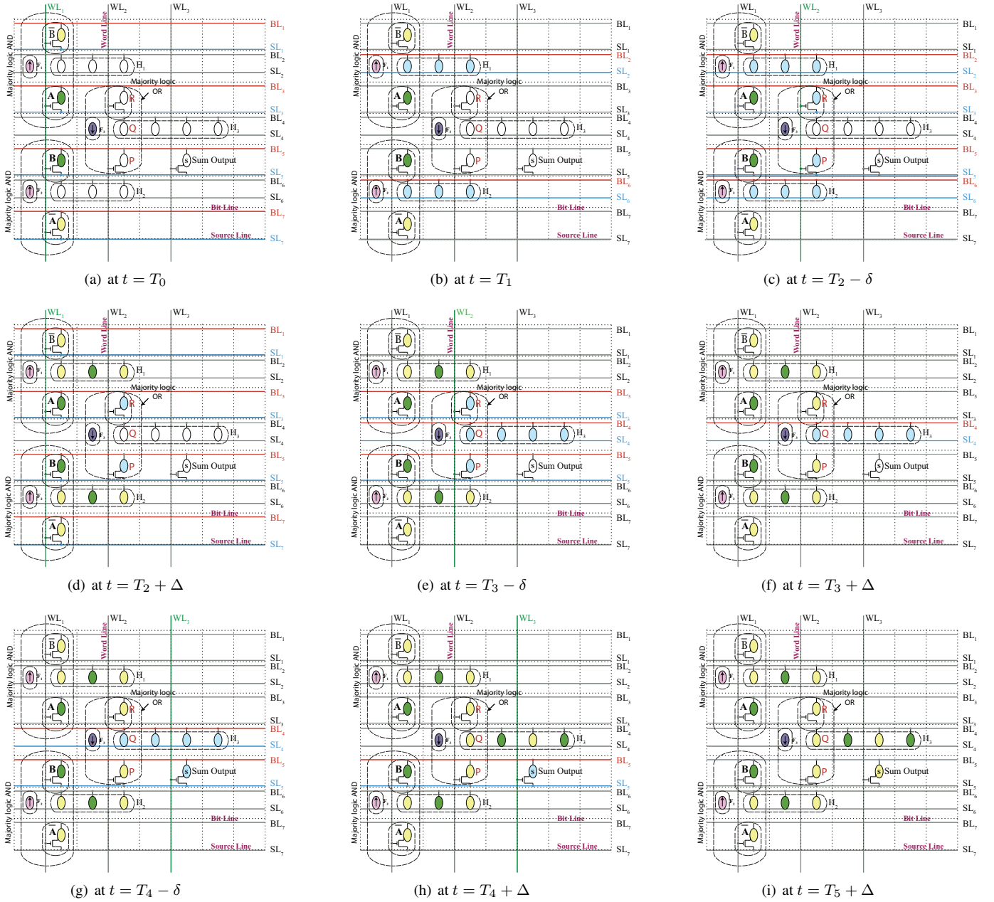
Figure 6: The sequence of logic flow through the architecture during the computation of Sum Output of a Half Adder. In the figures, green represents logic 1 , yellow represents logic 0 , blue represents the clocked state of a cell. The pink and the purple cells in the figure are the fixed cells storing logic 1 and logic 0 respectively. \delta and \Delta are positive quantities. \delta indicates the time to clock the MTJ while \Delta indicates the time taken by the MTJ to precess and settle down after the clock is released. when a potential difference is applied across the bit and source lines of a row, the lines are represented by red and blue. When a word line is selected, it is shown in grey.
