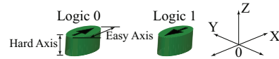
Figure 1: Single layer single-domain nanomagnets used in conventional magnetic logic. Logic 0 and logic 1 are denoted as the magnetization along the +x and -x direction respectively. The easy axis is aligned along the x direction. It is the energy minimum configuration of the magnet while the hard axis which is along the shorter dimension, represents the energy maxima or unstable configuration of the nanomagnetic cell.
